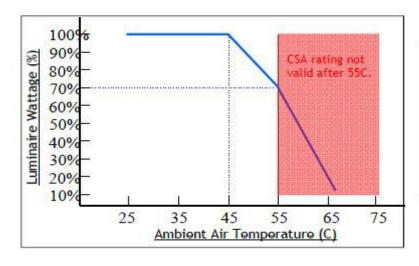
Control module activates at 45C. L70 output reached at 55C.
