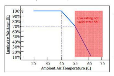
Control module activates at 45C. L70 output reached at 55C.
