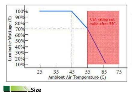
Control module activates at 45C. L70 output reached at 55C.
