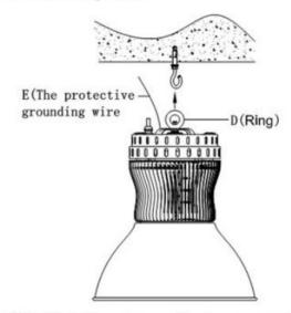
STEP No.4: Correct connection the power cable and E:
