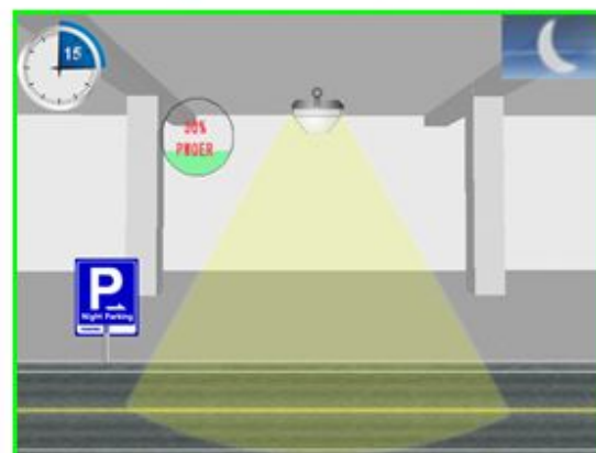
Mode 4: After a period people left(the period can be set), lighting brightness recover to 30%
