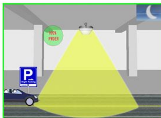
Model 2 : When people enter the sensing area, all lights will turn on (100%)
