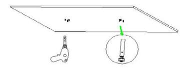
Step1: Drilled 6 holes with a 8mm diameter on the ceiling, please pay attention that the position of the hole should be aligned with screw holes on the product, holes distance please see installation instructions.
