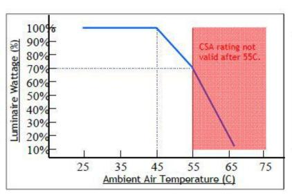
Control module activates at 45C. L70 output reached at 55C. Continuous operation after 55C with increased compensation. CSA certification valid to 55C only. Chart accurate for Standard Output versions only.
